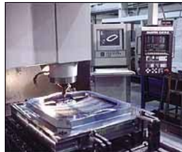
The Creative Evolution CNC, retrofitted to one of Reddog Industries' finishing mills, directs the machine's axis movements through finish machining of this container lid cavity. It was installed on a coexisting basis with the machine's original control.
