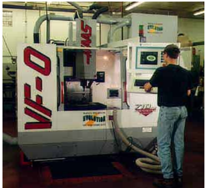
Barney Machinery Co.'s Evolution Series machining center, which combines the Creative Evolution CNC, a control developed specially for high-speed milling of 3D shapes, with the Haas vertical center, makes fast work of graphite electrodes at Chipsco Tools.
