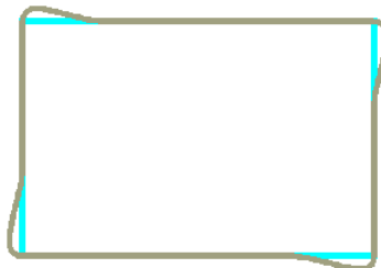
Fig. 5: Overshoots in corners of rectangular test
