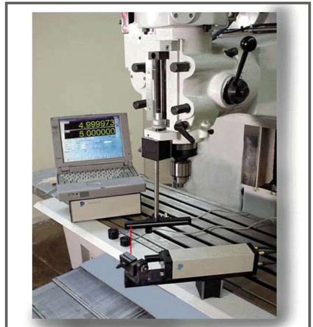
The Optodyne laser system not only calibrates machine axes for linearity, but also offers "ballbar" tests to check contouring performance.
