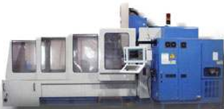
EPW's "new" Mazak AJV-60/120 Double Column Machining Center with Creative Evolution CNC
